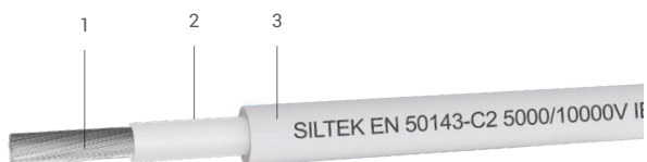
1. Rame flessibile Classe 5 CEI EN 60228 | Flexible copper Class 5 CEI EN 60228 • 2. Gomma siliconica EI2 | Silicone rubber EI2 • 3. Tipo D2 Mescola zero alogeni | Type c2 Halogen free compound
