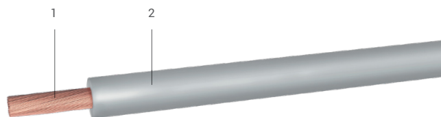
1. Rame flessibile ISO 6722 tipo A / tipo B | Flexible copper ISO 6722 type A / type B 2. Elastometro termoplastico base poliestere | Thermoplastic polyester elastomer TPE-E
